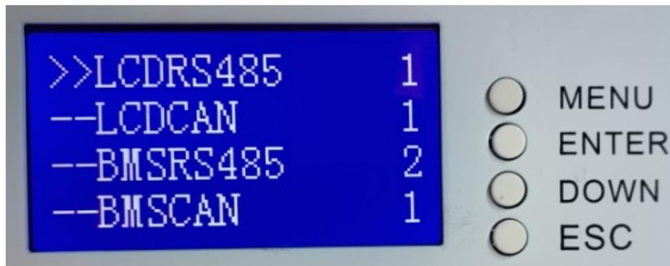
11.3 When you press the ENTER button, you will enter the LCD RS485 setting, as shown below:
