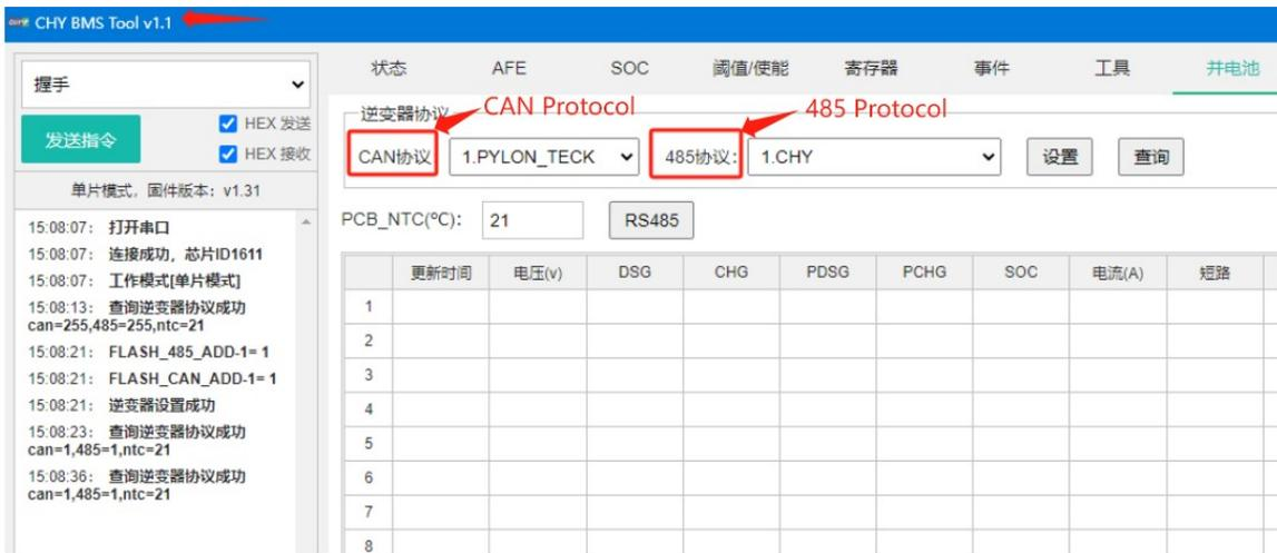
4.3 Select the corresponding inverter protocol from BMS Tool, click setting(设置),then restart the BMS ON/OFF , the inverter protocol will be set successful;
