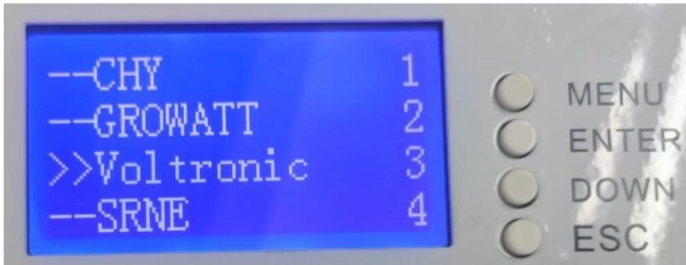
11.4 For instance, if you select "--Voltronic 3", press the Enter button, then press the ESC button. After three seconds, LCDRS485 and BMSRS485 will display the same number 3. This indicates that the setting change was successful, as shown below:
